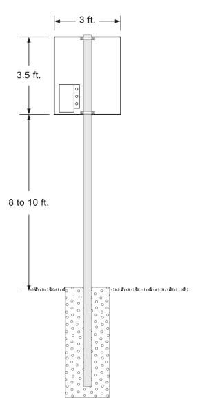
Once you have verified the position of the post and the size of the footing, you are ready to dig your hole, pour your concrete, and set your post. There are several techniques for ensuring proper alignment of the post. Typically installers will construct a temporary wooden support frame to hold the post in place while the concrete sets. Having a plumb post in the proper position is the key to a smooth mechanical installation.
