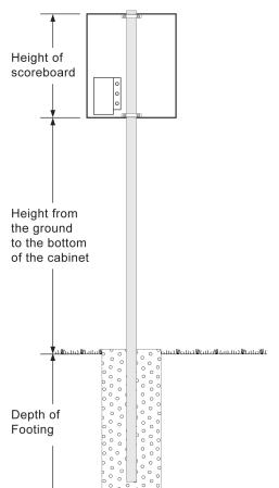
Post length is determined by the configuration of your display, its height above the ground, and the depth of your footing. Footing size is also related to the cabinet height and configuration. To some degree, the depth of the footing will be determined by the equipment available to the installer. In general, a smaller diameter hole needs to go deeper than a larger diameter hole. The trick is to create a footing hefty enough to provide stability for the sign structure.
